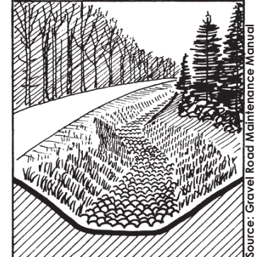
Use grass and stone to control erosion for ditches with more than 5% pitch.
