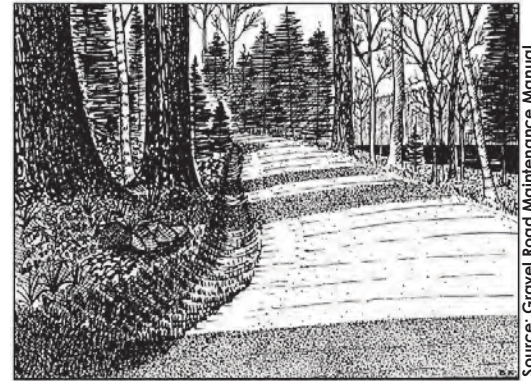
Crowned driveway with a rock-lined drainage ditch.
