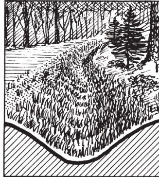
Plant grass to control erosion in ditches with less than 5% pitch.
